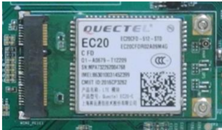
Figure 505: mini-PCIe Connector & 4G Module
