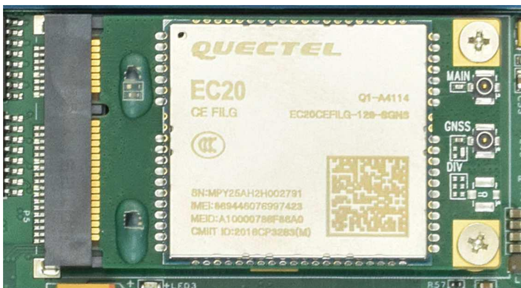
mini-PCle Connector & 4G/LTE Module
