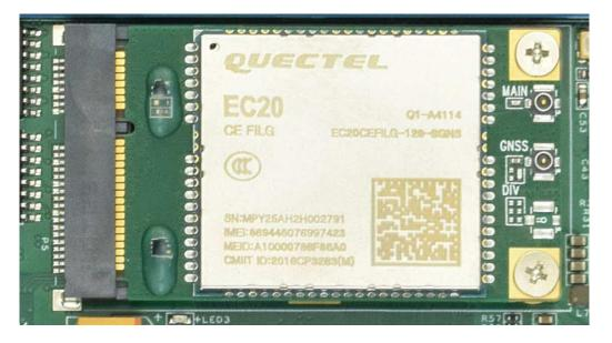
mini-PCIe Connector & 4G/LTE Module
