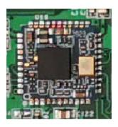
Figure 23: RTL8273 WiFi/BT Module
