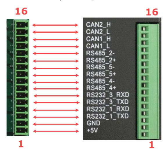
Figure 19: Serial pins connector
