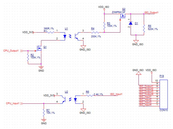
Isolated GPIO reduced schematic
