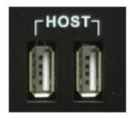
Figure 20: USB HOST Connectors (embedded/enclosed PC version)
