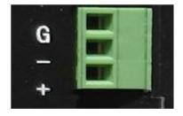
Figure 17: Power Input Section (embedded/enclosed version)
