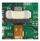
Figure 18: Figure 2: Capacitive Screen Connector
