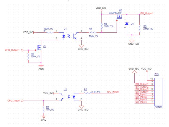
Isolated GPIO reduced schematic
