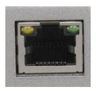
Figure 57: RJ45 LAN Connector
