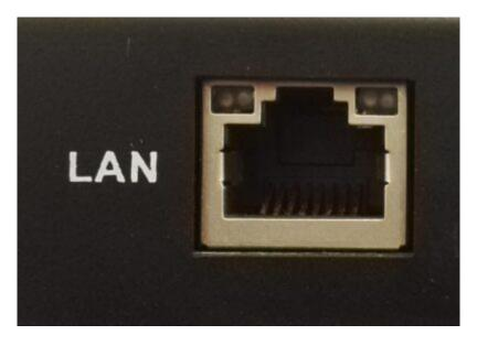
Figure 69: RJ45 LAN Connector
