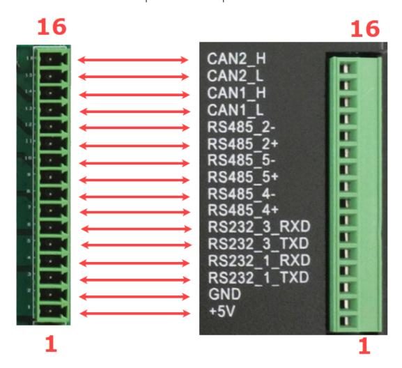
Figure 66: Serial pins connector
