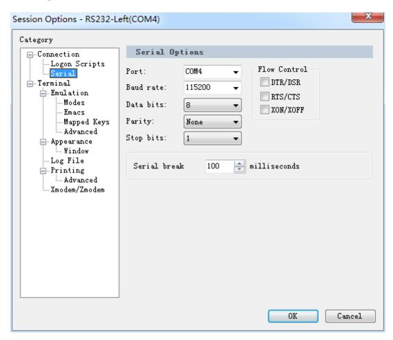
Figure 281: SecureCRT configuration
