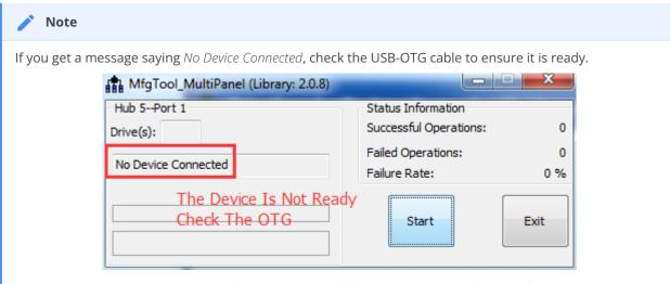
Figure 268: The USB-OTG cable is not connected correctly.
