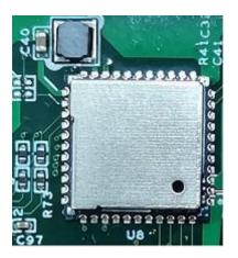
Figure 400: RTL8821CS WiFi/BT Module
