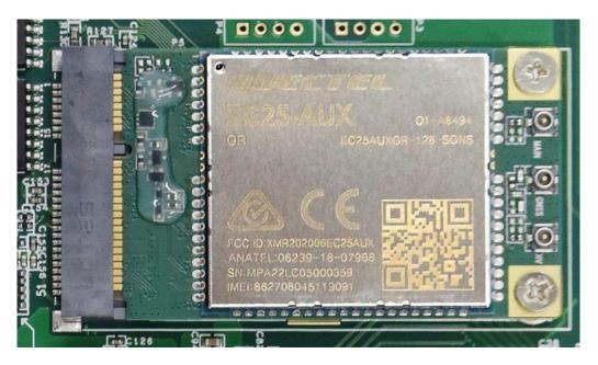
*mini-PCle Connector & 4G/LTE Module*
