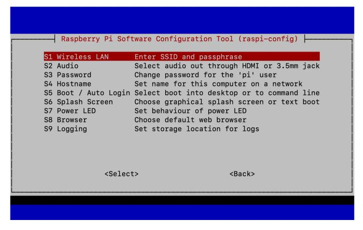
Method 2: Connecting WiFi from raspi-config TUI's System Options -> S1 Wireless LAN
