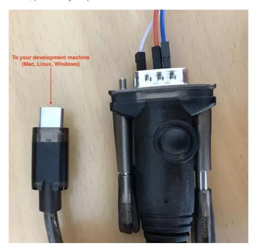
Use a USB to Serial Cable to Connect the Chipsee Industrial PC with Your Workstation
