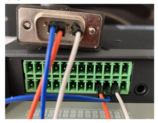
Connect 3 Pins with Dupont Wires (or with a phoenix connector)
