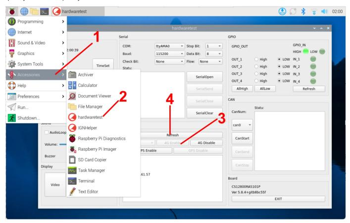
In the Hardware Test program, click *4G Enable*, then *Refresh* to check your connection information, you can also open the browser to test you're connected to the Internet.
